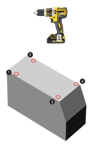
**4-** Remove the box from the bike and turn it upside down. Drill 4 holes Ø8 mm on the position of the marks made previously on the box.
