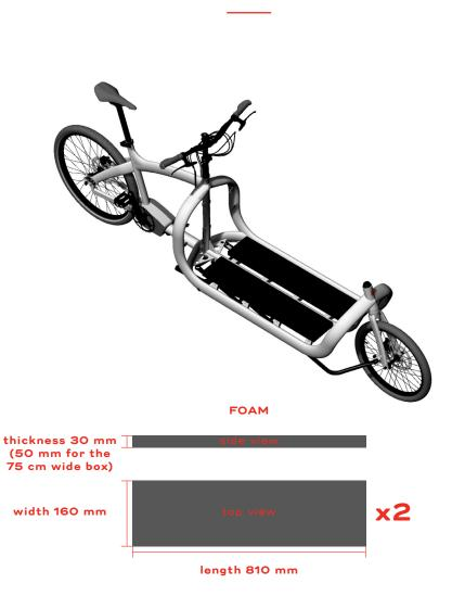
**1-** Using double sided tape, place two 30mm (50mm if the box is 75 cm wide) thick foam panels on the bike frame, as shown in the picture. The holes for the M6 bolts, close to the side tubes, have to stay uncovered. If the foam is missing, just use 4 pieces of wood, 30x30x810 mm (50x30x810 mm if the box is 75 cm wide) placed at the borders of the foam.
