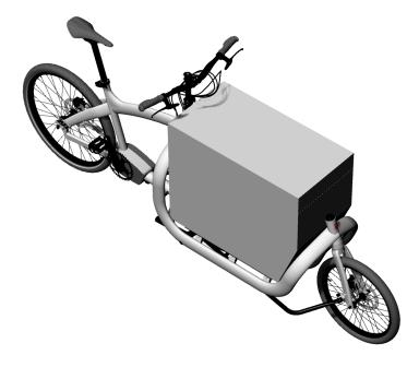
**2-** Place the flight case box on the foam panels, the distance between the headset and the rear part of the load deck has to be the same.
