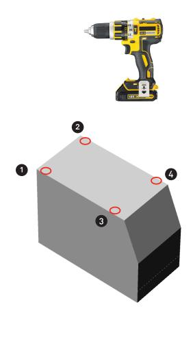
**3-** Using a long and thin marker, mark the center of the holes with the red circle on the bottom of the flight case box. The marker has to enter from the bottom of the frame.
