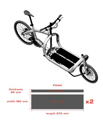
**1-** Using double sided tape, place two 30mm thick foam panels on the bike frame, as shown in the picture. The holes for the M6 bolts, close to the side tubes, have to stay uncovered. If the foam is missing, just use 4 pieces of wood, 30x30x570 mm, placed at the borders of the foam.
