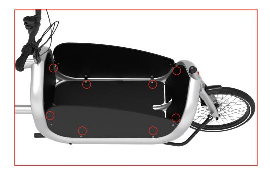
**3-** Tighten again the bolts on the rear, bottom and rear panels, in a firm way.
