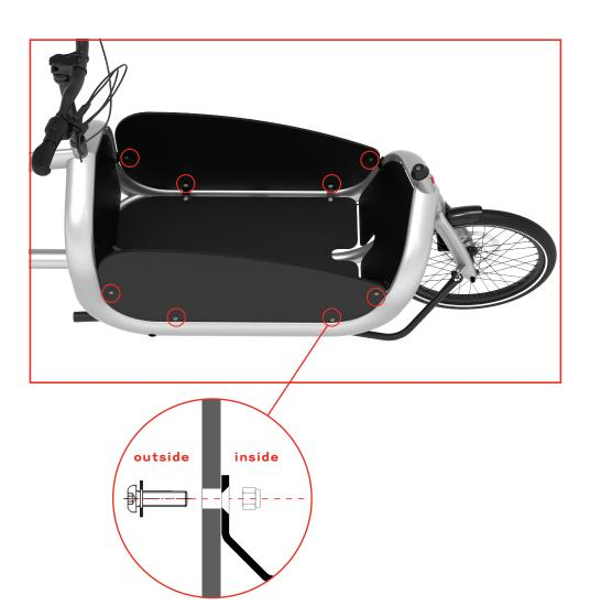
**2-** Connect the side panels to the brackets: bolt heads (with integrated washers) on the outside, nuts on the inside. Tighten firmly.
