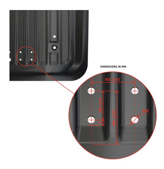
**3-** With a 9mm tip, drill 4 holes as shown in the picture. They have to stay in the middle of the flat part between the fins.
