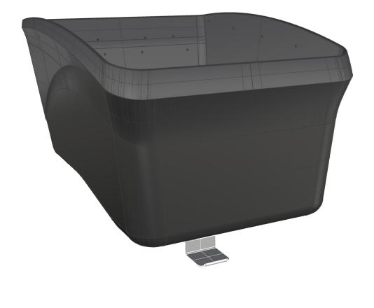
**3-** Connect the step in to the box using 2x DIN912 M6x40 bolt on the front and 2x DIN912 M6x45 on the rear. Put washers between the bolt head and box floor.
