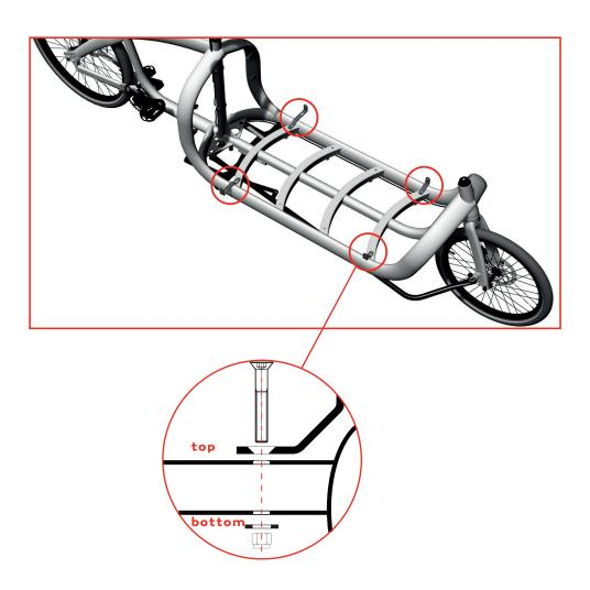
**2-** Place the brackets **B** and **C** on the frame, then put the bottom panel over them. The frame, panel and brackets holes have to match. Fix everything using bolts **#3** + nuts and washers on the back side.
