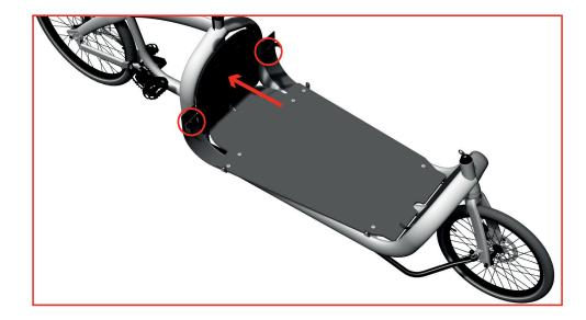
**3-** Place the extension panels as shown in the picture. Fix them on the bottom of the external hole of brackets **C** with bolts **#4** + nuts and washers.
