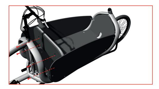
**5-** Mount the side panels connecting them to all the brackets using bolts **#2** + nuts.
