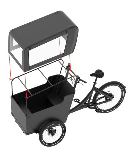
**4-** Take the 3 short straight bars and fix them to the side frame tubes with the 6x DIN7380 M6x25 bolts. The longer goes to the front, the shorter goes to the rear.
