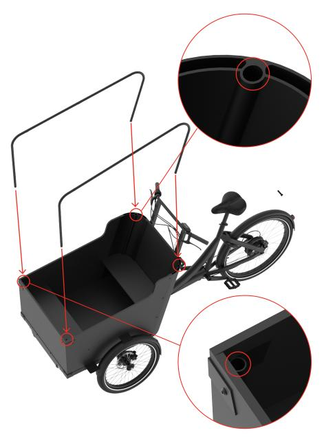
**3-** Insert the hood frame on the bike box: the frame has to enter into the tubes marked with the red circles.
