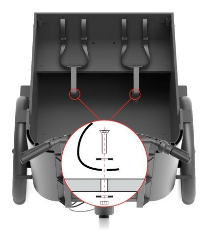
**4-** Connect seat belt bottom parts to the box floor, using 1xM6x25 bolt each in the specific threaded holes. Put bolts, washers and nuts according to the picture. **USE A TORQUE OF 5 Nm MAX.**
