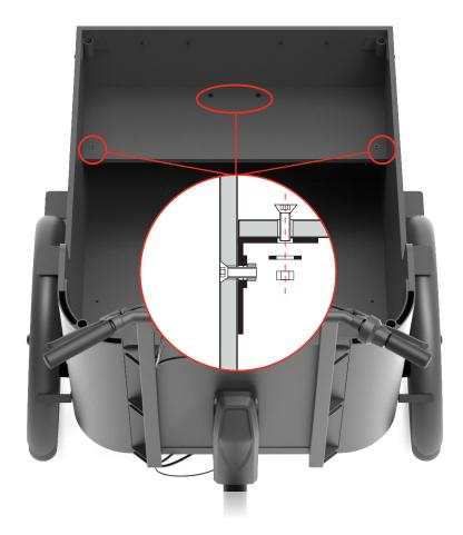
**2-** Place the front seat on the brackets, aligning the holes. Mount the seat on the brackets using 1x M6x25 bolt for each side bracket, and 2x M6x25 bolt for the front one. Put bolts, washers and nuts according to the picture. **USE A TORQUE OF 5 Nm MAX.**
